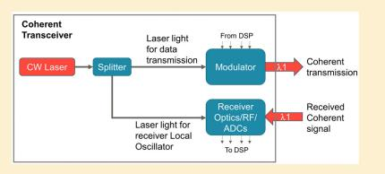
However, for BiDi applications in which the transmit and received wavelengths are different, the LO should not be derived from the transmission laser. A separate second laser is required as the LO. Thus, a coherent BiDi module contains dual lasers, one used to transmit the data, while the other is used as the LO. This allows the transmit wavelength to be independent from the receive wavelength.
