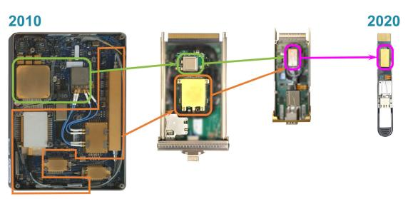
Figure 10. Evolution of coherent module size over time.
