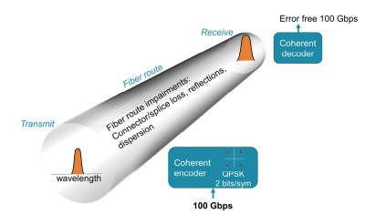
*Figure 7. Error-free coherent transmission of 100Gbps QPSK modulation example, tolerant to multiple impairments (only one transmission direction shown).*
