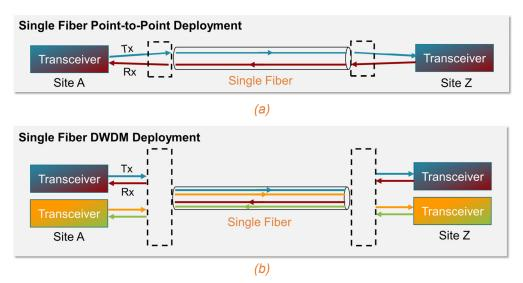
Figure 5. Optical transmission in a service provider edge/access network over (a) a single fiber BiDi link and (b) a DWDM single fiber BiDi link—in both cases, the transmit wavelength is different from receive wavelength for each data transmission stream. The optical implementation to combine signals into a single fiber depends on the link requirements.
