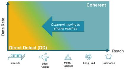
Figure 6. Coherent solutions are evolving towards shorter reaches.
