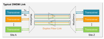
Figure 4. Typical DWDM link which may or may not be amplified.
