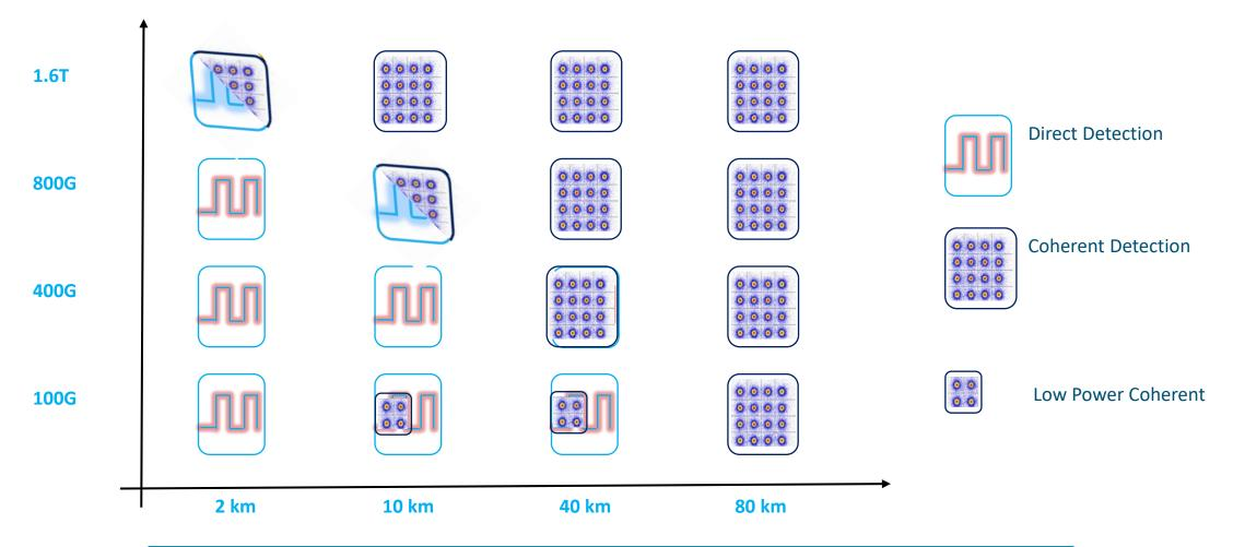
**Low Power Coherent 100G Replacing Nx10G in Short Reaches**
