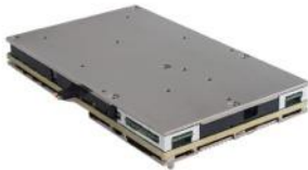
1.2T Coherent Module (AC1200)
